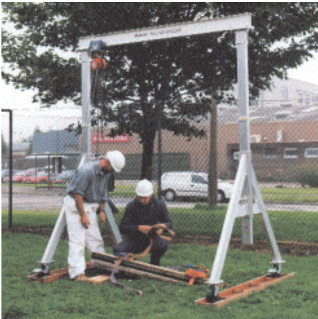
Illustration 3. Preparing to lift a stone – the use of soft strops.
